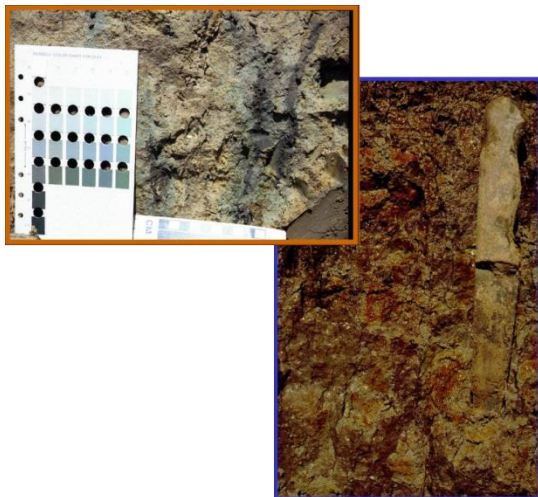
Figure 7 Photographs of mottled soil, indicative of waterlogged conditions
