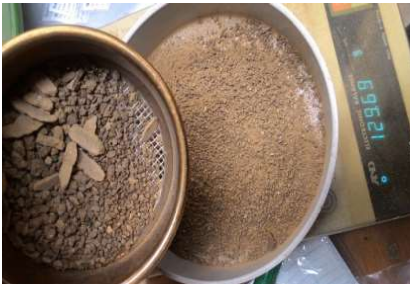
Figure 3.8 Hand sieving for aggregate samples size below 2mm (chemical portion)
