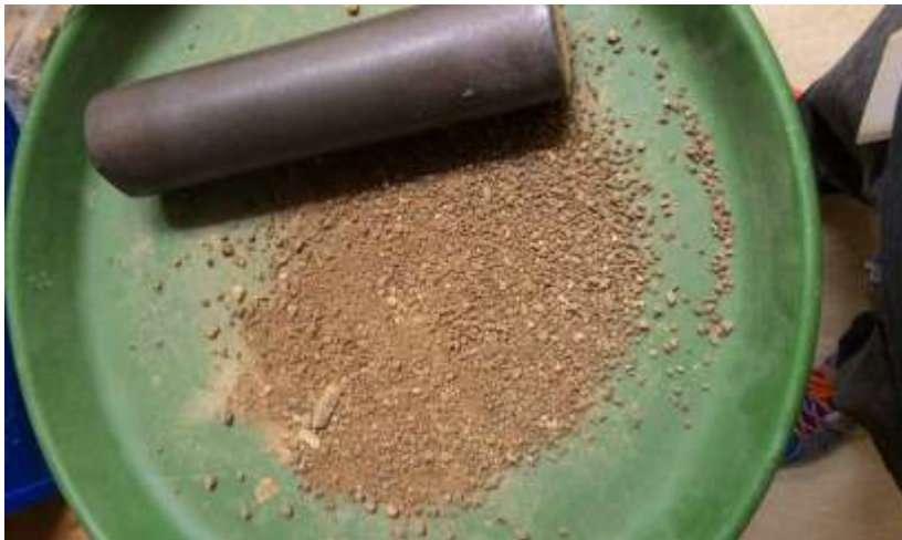
Figure 3.7 Ground aggregates were further broken-down by hand-crushing for chemical properties analysis with a metal pestle
