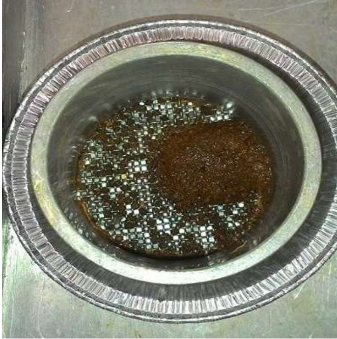
Figure 3.9 The aggregates that were above a trapped air bubble, could not pass through the sieve due to blockage of pathways. The aggregates assembled did breakdown by applied energy and the sizes were visually smaller than the sieve size (<1mm).
