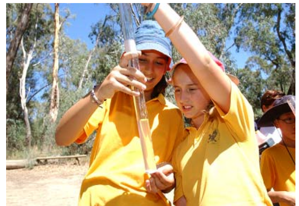
Testing Turbidity in the Goulburn River
