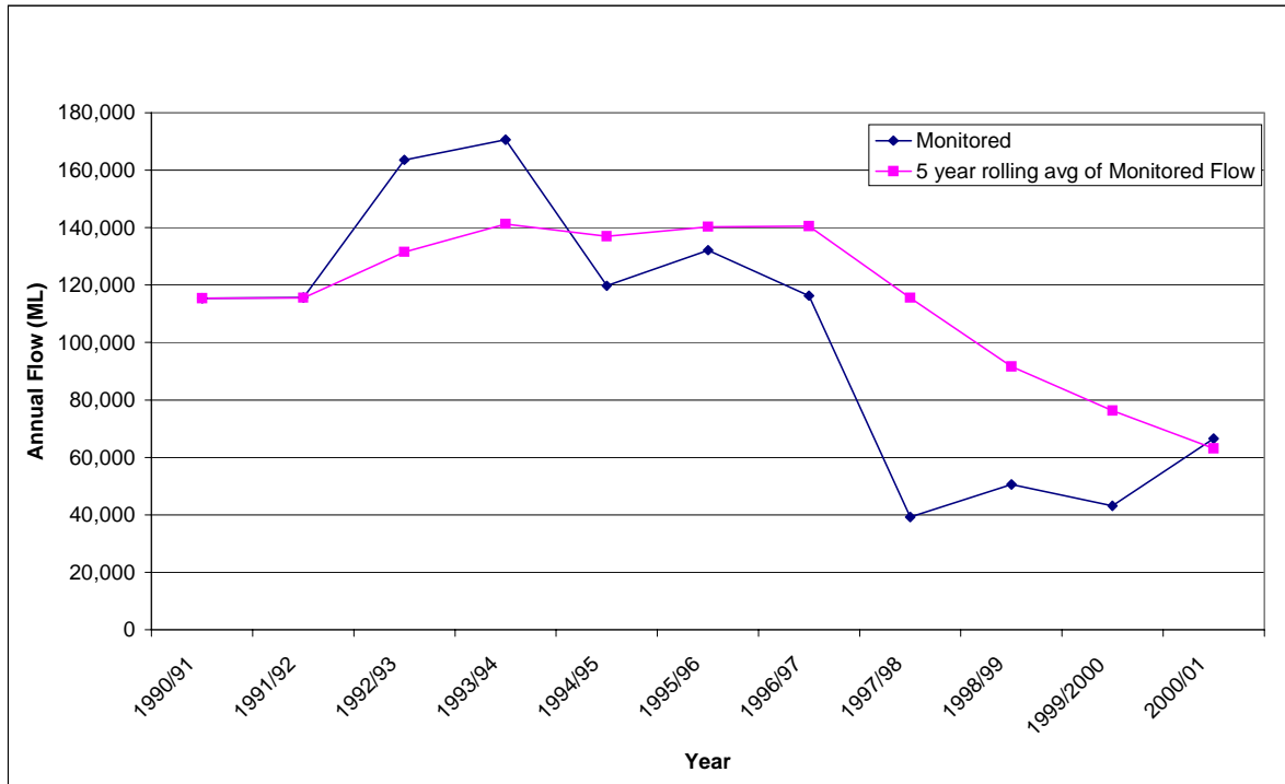
Figure 6 - Flow from Monitored irrigation drains (Deakin, Rodney, Toolamba, MV 6)
